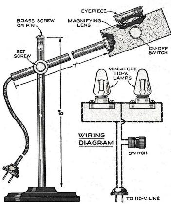
Extension arm adjusts for height and length, though the angle in relation to the stand remains fixed. Dimensions may be altered, if desired.
