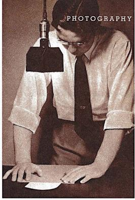
LEFT ABOVE: One of the most efficient safelight combinations: direct illumination 18 inches from tray and indirect general lighting 10 inches from wall. RIGHT ABOVE: Performing simple safelighttest on paper. BELOW: Paper and film sensitivity chart.
