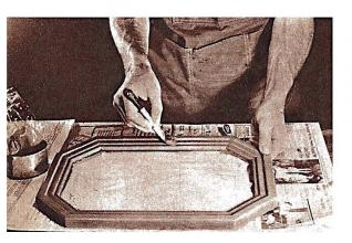
power scroll saw is not available, the plaque can be cut by hand. Use masonite or ¼" three-ply stock for the background, fitting it with a hanging tab, and stretch the velvet over the face, gluing the edges at the back. Attach the plaque with a brass escutcheon nail driven through the eye of the bird, so that it can be pried off for ease in cleaning the velvet.
