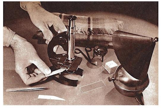
Inserting tapered cardboard strip between mirror and object will produce a darkfield effect to bring out surface detail of textiles.
