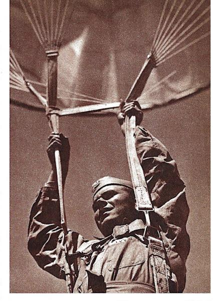
"Slipping" a chute to change the direction of its fall is simple. Just pull down on one side, as shown above, grasp the shrouds and let 'er slide. Below: The ways to "spill the wind." Either run around canopy to face the wind, or pull the bottom shrouds.
