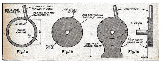
Pump case assembly is shown above. Be sure to make the base very rigid so there can be no vibration or working of the shaft.
