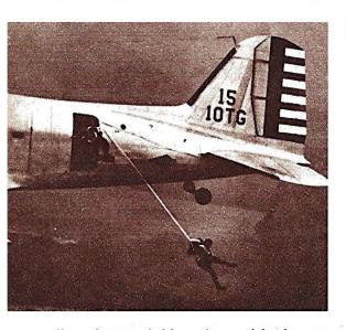
Above, the automatic 'chute release used by Army paratroopers—nothing more than a length of cable, seen in the photo—is about to pull the jumper's canopy out of its pack. And, at right, the 'chute is now opening. Below, the trooper, having landed, is pulling the lower shrouds to "spill the wind."
