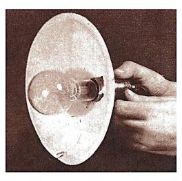
ABOVE: An emergency photo lamp reflector can be made very readily with the aid of a paper, picnic or pie plate as illustrated. Cut out a small pie-shaped segment of the plate and pull it together into cone-shape. Then cut a hole in the center large enough to take the electric lamp socket. The plate can be held together with a pair of paper clips.—Wm. Swallow
