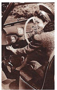
"Step-On" emergency brake, by Buick, operates by foot and has dash release to eliminate "fumbling."
