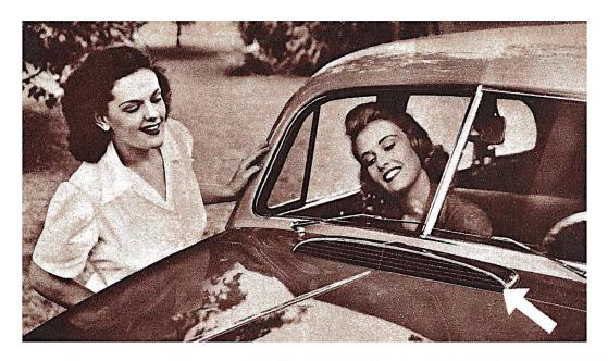
Cowl ventilators on the new cars are done away with or drastically changed. Here, above and at right, is the Nash "Weather Eye" system of air-conditioning, using fresh air for healing.
