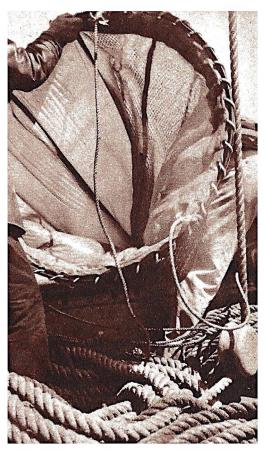
The net, its large iron hoop attached, is made ready for going over the side. The rig is especially built for dragging.
