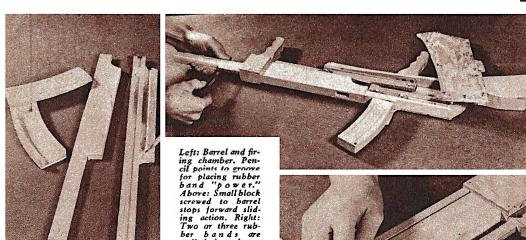
pulled in place with storepipe wire.
