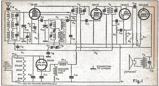
Cla, Clb—Gang Condenser, two sections, 365 mmf., each section, Meissner or Trutest C2, C4, C10, C11, C16—Aerovox tubular condensers, paper, .05 mfd., 400 volt, type 484 C3—Aerovox tubular paper condenser, 0.5 mfd., 400 volt, PARTS LIST C5, C12—Aerovox mica condensers, .0001 mfd. C6—Meissner mica condenser, .003 mfd., (part of padder kit No. 22-5202)
