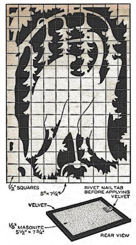
Above: Design of the plaque is laid out in half-inch squares for easy copying. Or you may wish to originate a picture yourself. Sketch it on thin paper, rub the back with black pencil and trace over it, for transferring to the board. Right:
