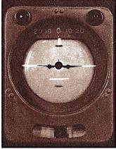
Functions of the Flightray are shown in the diagram at left, above. When the ship is off its course, the dial appears as at right, above. She's gaining speed, banking and too far left. Below, all white lines match black—she's in on the beam!
