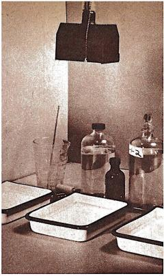
LEFT ABOVE: Examination of films (and prints) during development should be within specified time, and not too close to the safelight. RIGHT ABOVE: The safelight giving direct illumination should be at least 18 inches away from developing trays.
