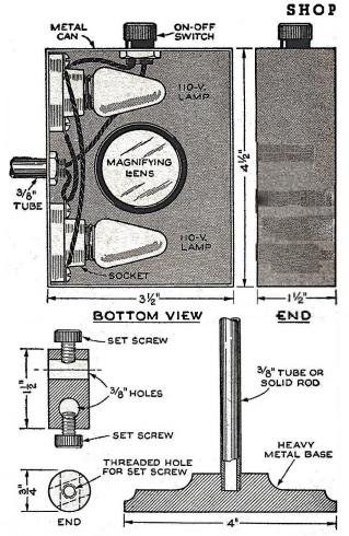
Top drawing gives bottom and end layouts of the box. Small sketch at lower left is cross-section of the adjuster piece, Stand goes through one 3/8," hole, arm through the other.
