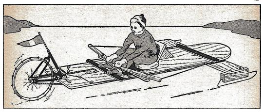
THE platform consists of a simple plank 9 ft. long, 18" wide and 1" thick. Or you can cleat two narrower boards together underneath, making due allowance for fittings, etc. Round off one end for the bow but leave the stern square.
