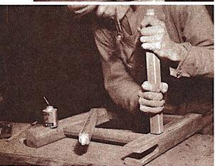
Above: Fitting a side together. Slot in leg is for front wheel. Right: To insure perfect centering of the wheel holes a hole is first bored in wood block and tested over snug dowel with tail stock brought against it.
